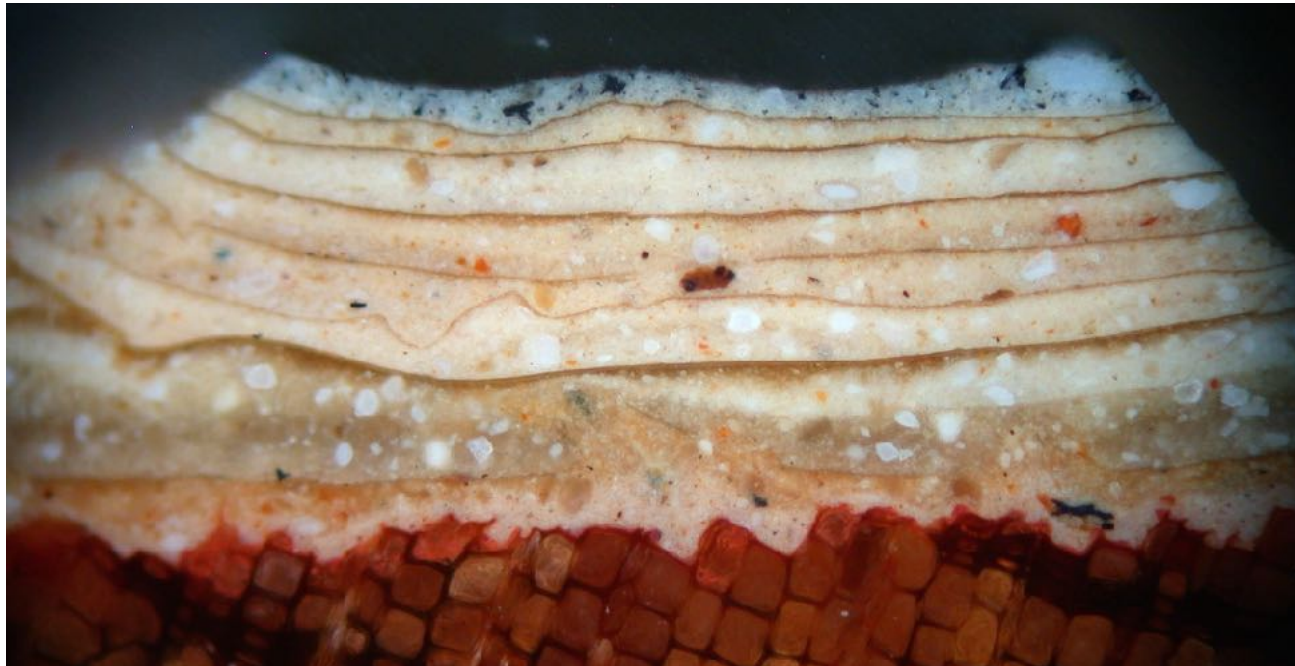
Sample 150 (fragment 2) showing the earliest paint schemes and timber substrate. The sample is from panelling on the ground floor near front door of 5 Tower Green photographed in dark- field light at 200× magnification. Printed magnification not calculated.
