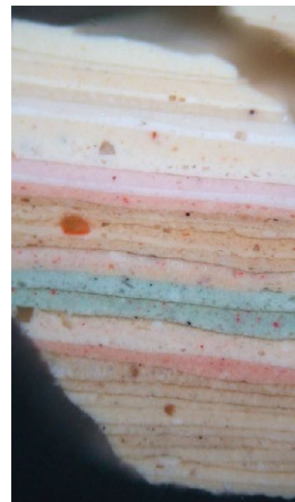
Above centre: Sample 59 (from chimney breast in main first-floor room, house 4) – detail of sample photographed in cross-section under dark-field reflected light at 200× magnification; above right: Sample 59 photographed in cross-section under dark-field reflected light at 200× magnification. Printed magnifications not calculated.
