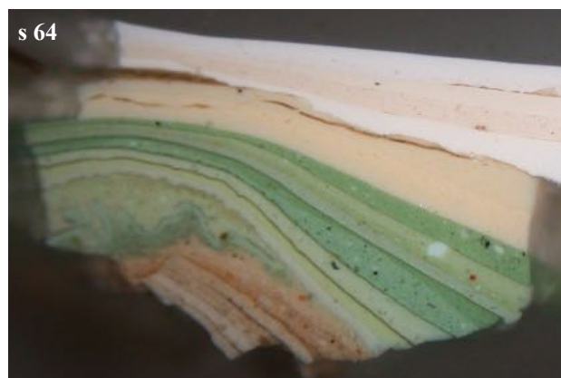
Above left: Sample 64 photographed in dark-field reflected light at 100× magnification; above centre: As before after staining for lead with potassium chromate; above right: Sample 64 after staining for lead with potassium chromate under UV illumination with Leica filter cube A. Printed magnifications not calculated.
