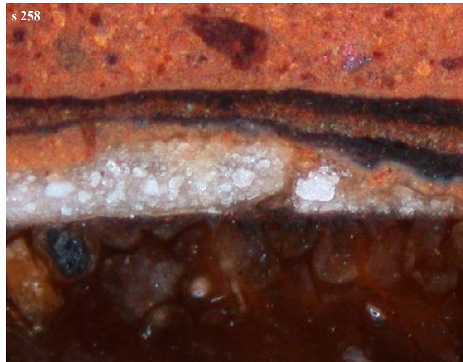
Above left: Sample 258 location; above right: Sample 258, photographed in cross-section under dark-field reflected light at 500× magnification (printed magnification not calculated).
