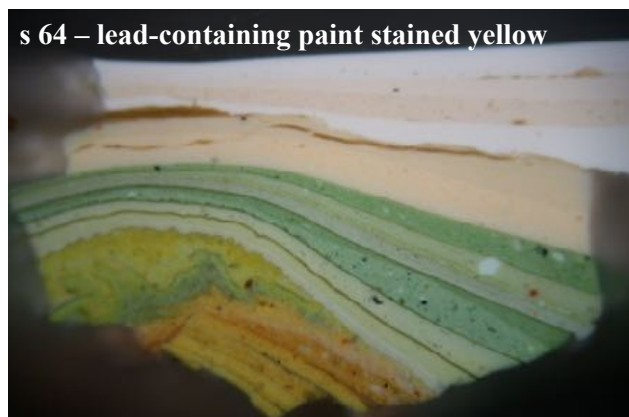
Above left: Sample 64 photographed in dark-field reflected light at 100× magnification; above centre: As before after staining for lead with potassium chromate; above right: Sample 64 after staining for lead with potassium chromate under UV illumination with Leica filter cube A. Printed magnifications not calculated.
