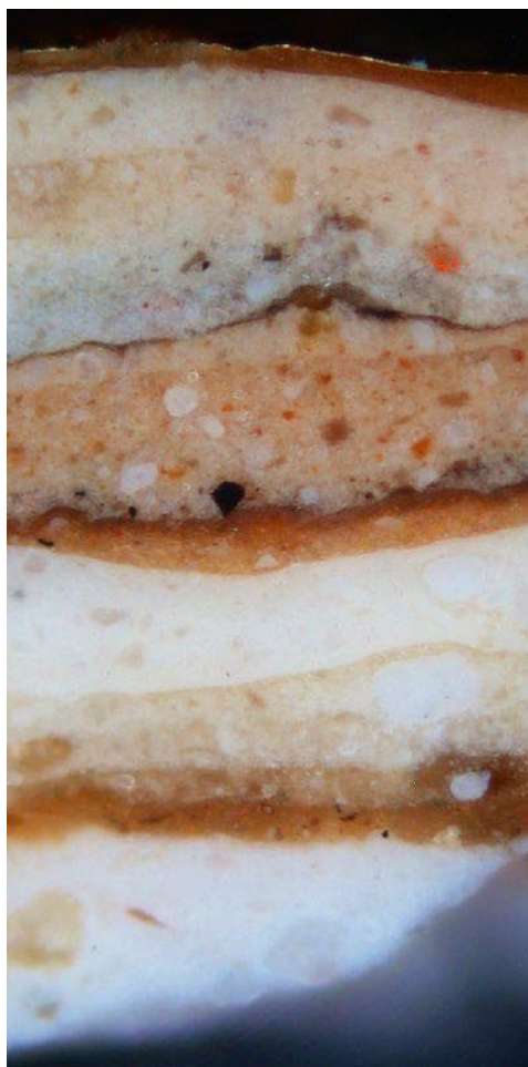
FIG. 27 Cross-section sample from volute leaf tip of north-east Corinthian capital, photographed under darkfield reflected light (2016/54). 200× magnification at capture; printed magnification not calculated.
