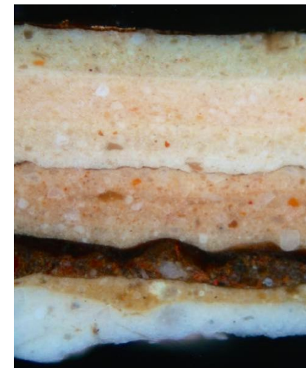
FIG. 26 Cross-section sample from the 'weak' foliate pattern on the anthemion fascia, photographed under darkfield reflected light (2014/22). 200× magnification at capture; printed magnification not calculated.
