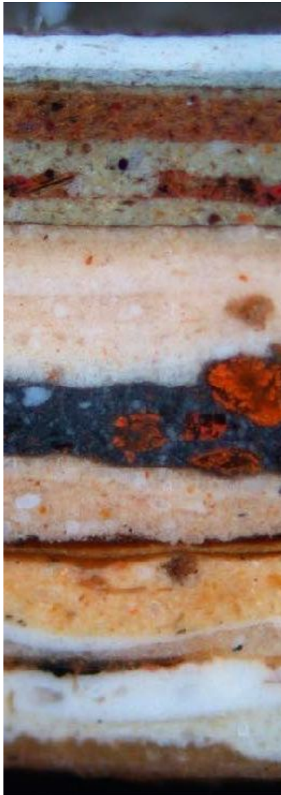
FIG. 22 (right) Cross-section sample from the fillet moulding on the north-wall architrave, adjacent to uncovering, photographed under darkfield reflected light (2016/ 44). 200× magnification at capture; printed magnification not calculated.
