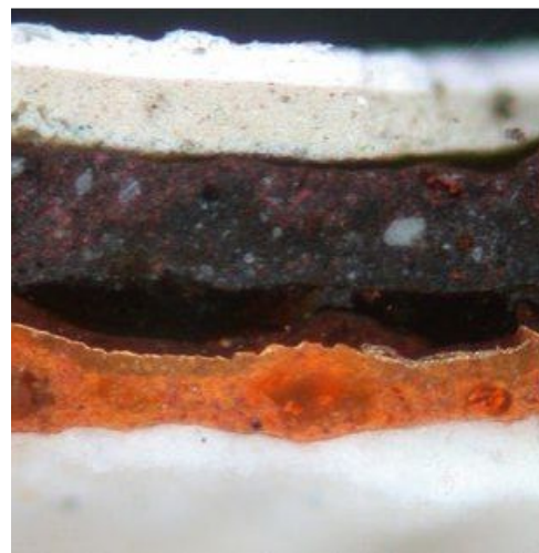
FIG. 10 Cross-section sample from the curved planceer at the northern end of Minerva photographed under darkfield reflected light (2016/30). 200× magnification at capture; printed magnification not calculated.
