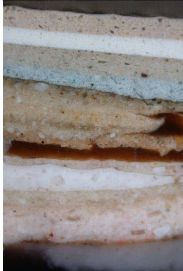
FIG. 28 Cross-section sample from wall-frieze background, east wall, photographed under darkfield reflected light (2016/5). 200× magnification at capture; printed magnification not calculated.
