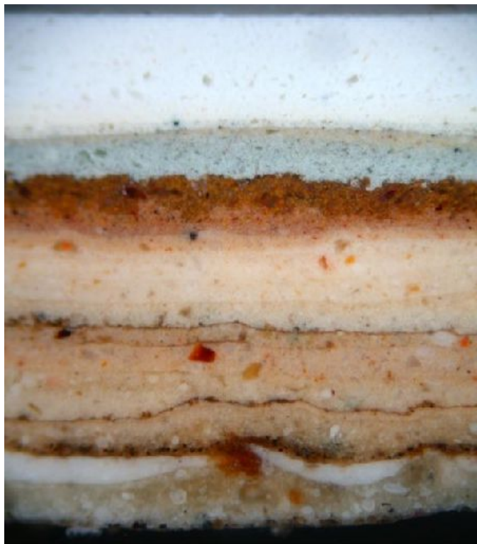
FIG. 33 Cross-section sample from the bead moulding of the entablature, photographed under darkfield reflected light (2014/26). 200× magnification at capture; printed magnification not calculated.
