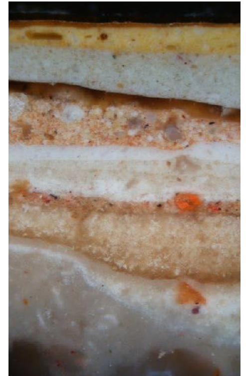
FIG. 29 (below) Cross-section sample from eyebrow of east-bay mask wall frieze, north wall, photographed under darkfield reflected light (2016/5). 200× magnification at capture; printed magnification not calculated.
