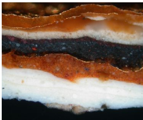
FIG. 14 Cross-section sample from small cyma reversa between spandrel caisson and rectangular section of planceer, north-east ( Minerva ) section, photographed under darkfield reflected light (2014/16). 200× magnification at capture; printed magnification not calculated.
