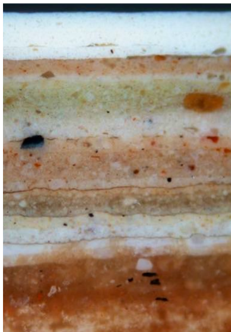
FIG. 31 Cross-section sample from the window reveal of the northernmost window at the first-floor level, photo-graphed under darkfield reflected light (2014/34). 200× magnification at capture; printed magnification not calculated.
