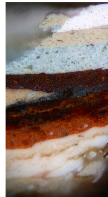
FIG. 17 Cross-section sample from vertical edge of guilloche edge band near Apotheosis , photographed under darkfield reflected light (2016/9). 200× magnification at capture; printed magnification not calculated.
