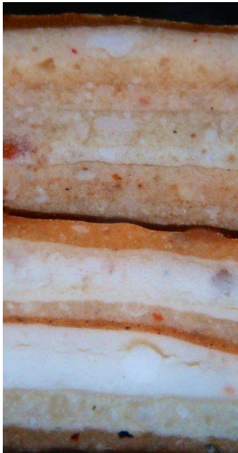
FIG. 23 (below) Cross-section sample from the cyma revers moulding above the entablature frieze, photographed under darkfield reflected light (2016/ 48). 200× magnification at capture; printed magnification not calculated.
