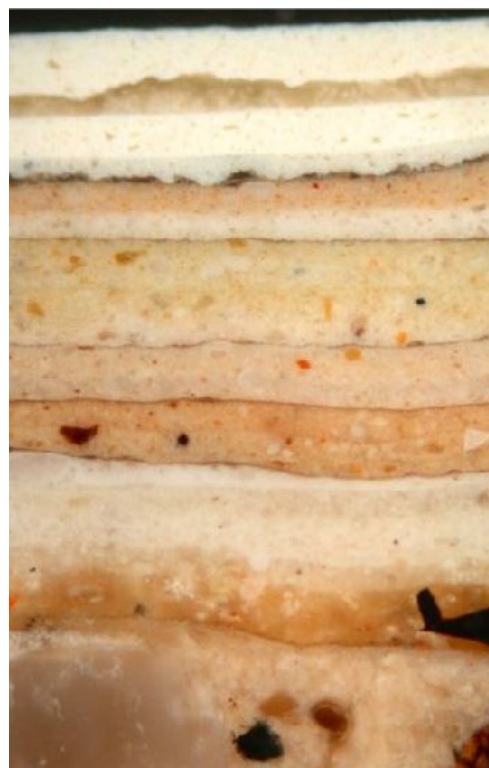
FIG. 32 (below) Cross-section sample from the south-side, ground-floor window reveal of the second-from-north west-wall window, photographed under darkfield reflected light (2014/34). 200× magnification at capture; printed magnification not calculated. A thick layer of dirt is visible between the late-19th-century paint and the modern schemes, possibly indicating damage to the window during WWII.
