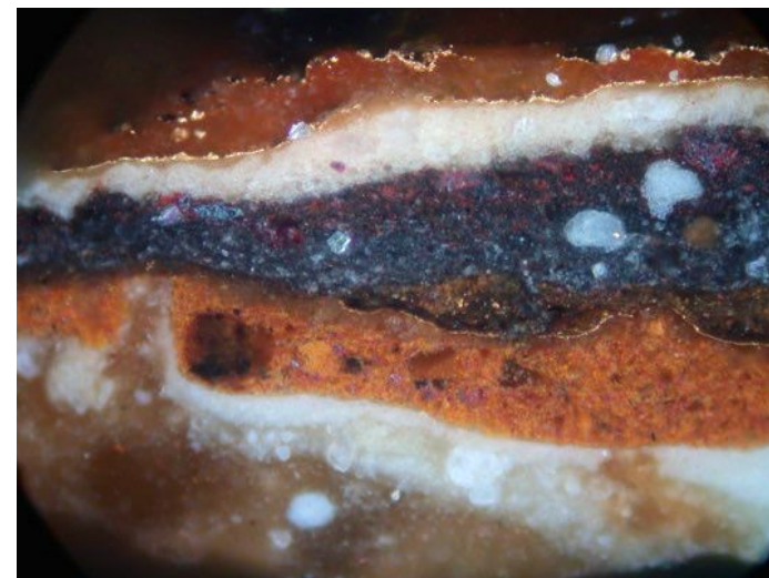
FIG. 15 Cross-section sample from arris of gilded frame around Minerva , north end, photographed under darkfield reflected light (2018/14). 500× magnification at capture; printed magnification not calculated.
