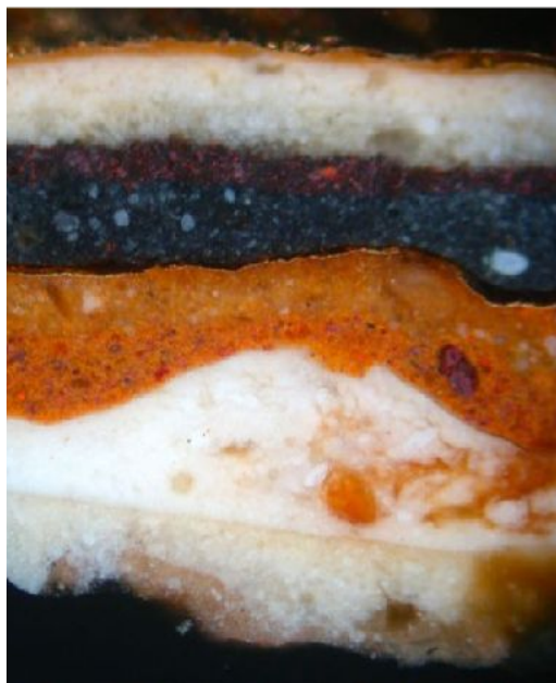
FIG. 18 Cross-section sample from waterleaf and dart moulding of coffer adjacent to Hercules , photographed under darkfield reflected light (2014/12). 200× magnification at capture; printed magnification not calculated.
