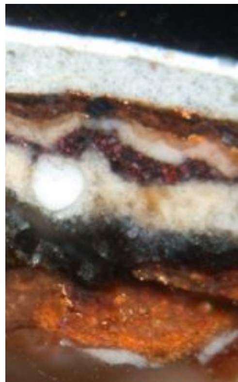
FIG. 16 Cross-section sample from vertical edge of guilloche edge band at south end of ceiling, photographed under darkfield reflected light (2016/8). 200× magnification at capture; printed magnification not calculated.
