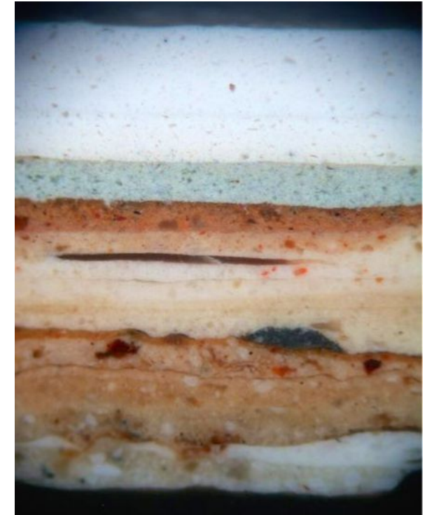
FIG. 30 Cross-section sample from baluster of east-side balcony, photographed under darkfield reflected light (2018/38). 200× magnification at capture; printed magnification not calculated.
